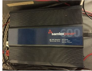
Inverter Samlex Power DC-AC Inverter: 600 W
